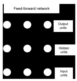
**Figure 1** A standard feed-forward network containing three layers of units. Information flows bottom-up from input to output units. These types of networks are normally trained using the back-propagation algorithm, which minimizes the discrepancy between the network's actual and desired output.
